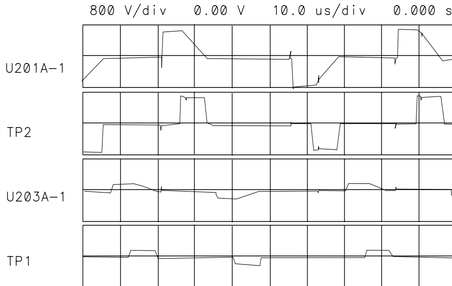
Figure 10-9 Normal X/Y Line Generator Waveforms
